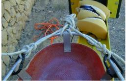
an end to end "Inline" pull. The CTM200 if placed in an end to end "Inline" pull. The CTM200 was placed in the SPD and rigged with a 3 point inline litter harness as specified by the Technical Rescue Riggers Guide published by Rick Lipke. The litter harness was constructed of 11mm static Kernmantle rope.
