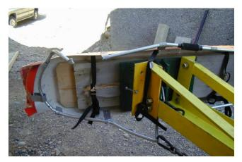
the bracket closest to the carabiner. At this point, the litter, while badly damaged was still attached to the litter harness by three of four attachment points. After several more seconds it was determined the litter had sustained enough damage to render it inoperable. Absolutely no damage was done to the <sup>1</sup>Fastlock<sup>TM</sup> System and the remnants of the litter were disassembled at the completion of the test.
