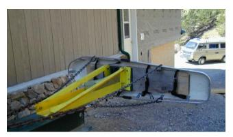
A rigid backboard was manufactured to place in the bottom of the litter to distribute the load of the SPD across the length of the litter. The footprint of the backboard was 60 inches by 11.25 inches. The distance from the center of the ram to the end of the litter was 47.25 inches and from the head of the litter to the ram was 34.75 inches.
