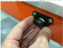
8. Place the washer (6) over the stud on the inside of the sled and then thread the Flexlock Nut (5) onto the end of the stud and tighten.
