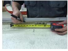
On the Left side of the toboggan, measure back 34 3/4" from the forward most Footman Loop and make a mark in the inside of the toboggan. This will be the location of your rear Slide Arrest Anchor on the Left side.
