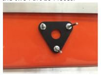
5. Drill a 5/8" hole through the toboggan in the center of Part 10.
