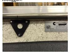
4. Place the second Part 10 on the outside of the toboggan and align the holes you drilled in Step 3. Insert three 3/16ths inch rivets through the holes in Part 10 on the outside of the toboggan, through the toboggan and then through the second Part 10 on the inside of the
