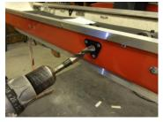
4. From the outside of the toboggan, insert the threaded stud (7) that protrudes from the Anchor Spike Sleeve (3) into the hole, seating the Delrin Bearing into Part 10 and into the hole.
