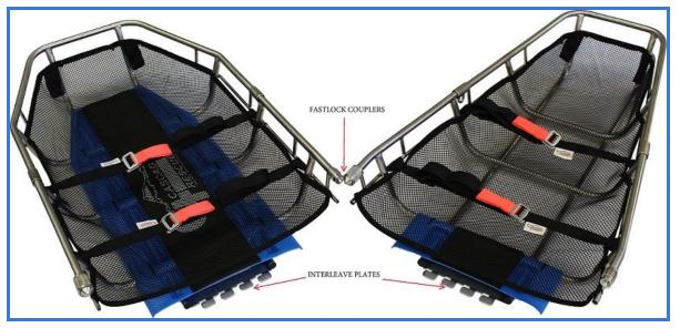
Two-Piece Litters have a rapid take-down FastLock System comprised of (2) FastLock Couplers and a two-part Interleave Plate.
