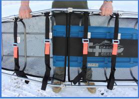
Use slight pressure to lift one section of the litter straight up, while pushing down slightly on the other section. This will engage the tabs of the Interleave Plate (3). Rotate the ends of the litter away from you until the litter is relatively flat and the FastLock Couplers engage (4).
