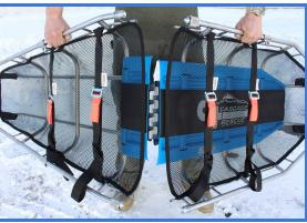
To assemble: Pick up the litter and bend in the middle, pulling toward you, until the litter is at an approximately 30 degree angle (1). Insert the tabs on the Interleave Plate through each other (2).
