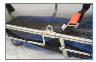
Cascade Rescue Company's patented ALPs allow a variety of litter rigging to be used. Position them straight up and use them with a traditional four point harness or rotate them to the outside to facilitate use with a two point harness for vertical work. When not needed, simply fold them in the down position and they are completely out of the way with no potential for patient injury. Each ALP has a MBS of 9kN.
