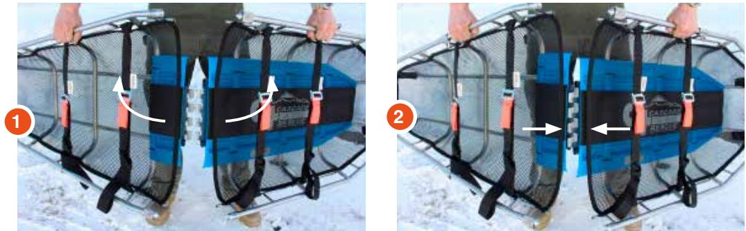
Use slight pressure to lift one section of the litter straight up, while pushing down slightly on the other section. This will engage the tabs of the Interleave Plate (3). Rotate the ends of the litter away from you until the litter is relatively flat and the FastLock Couplers align (4).
