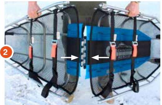
Use slight pressure to lift one section of the litter straight up, while pushing down slightly on the other section. This will engage the tabs of the Interleave Plate (3). Rotate the ends of the litter away from you until the litter is relatively flat and the FastLock Couplers align (4).
